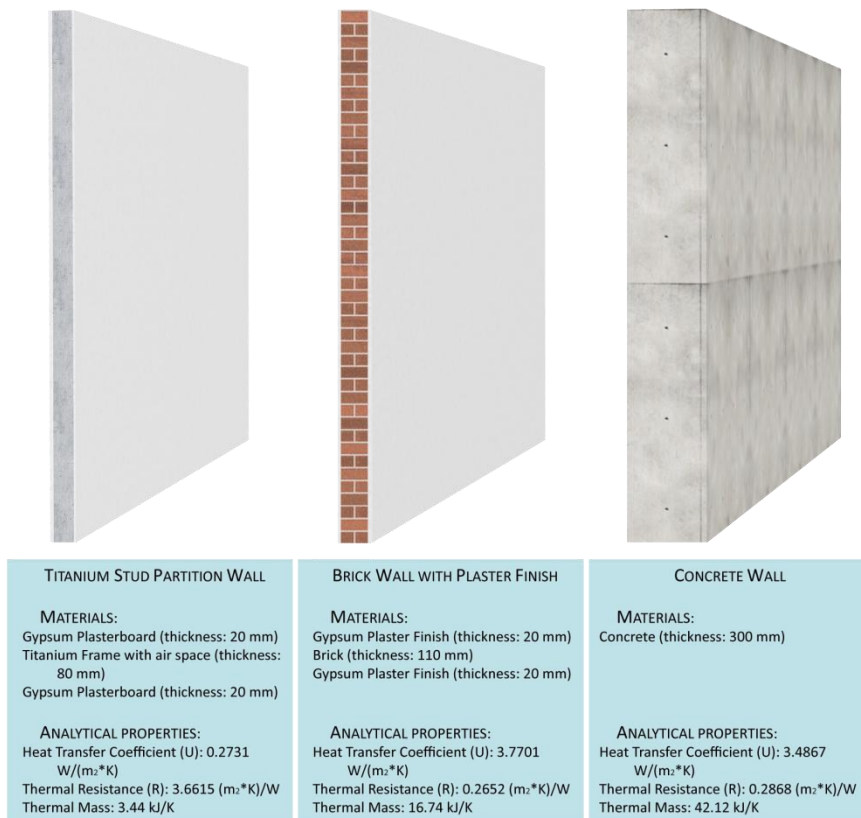
Figure 9.06 – Material and analytical properties contained in three different variations of the same wall.
