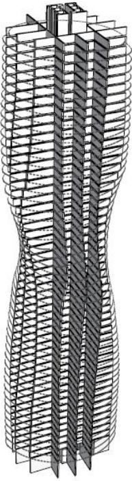
Figure 8.12 – Structural Diagram of the AWTs. The walls adapt themselves to the rotation of the tower in each floor. (source: Lagendijk et. al, 2012)
