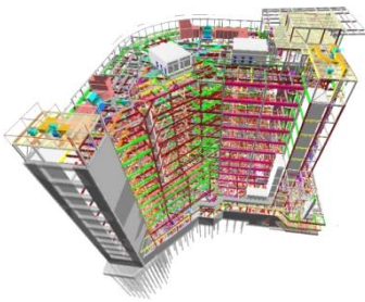
Figure 3.01 – A BIM model containing all relevant data needed to digitally simulate the process of building. (source: http://national-cba.com/ )
