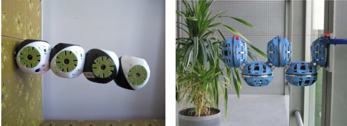
Figure 3.1: Module displacement of (Left) two Roombot modules and (Right) five ATRON modules caused by gravity: (Courtesy of BioRobotics Laboratory, EPFL and Østergaard et al. (2006))
